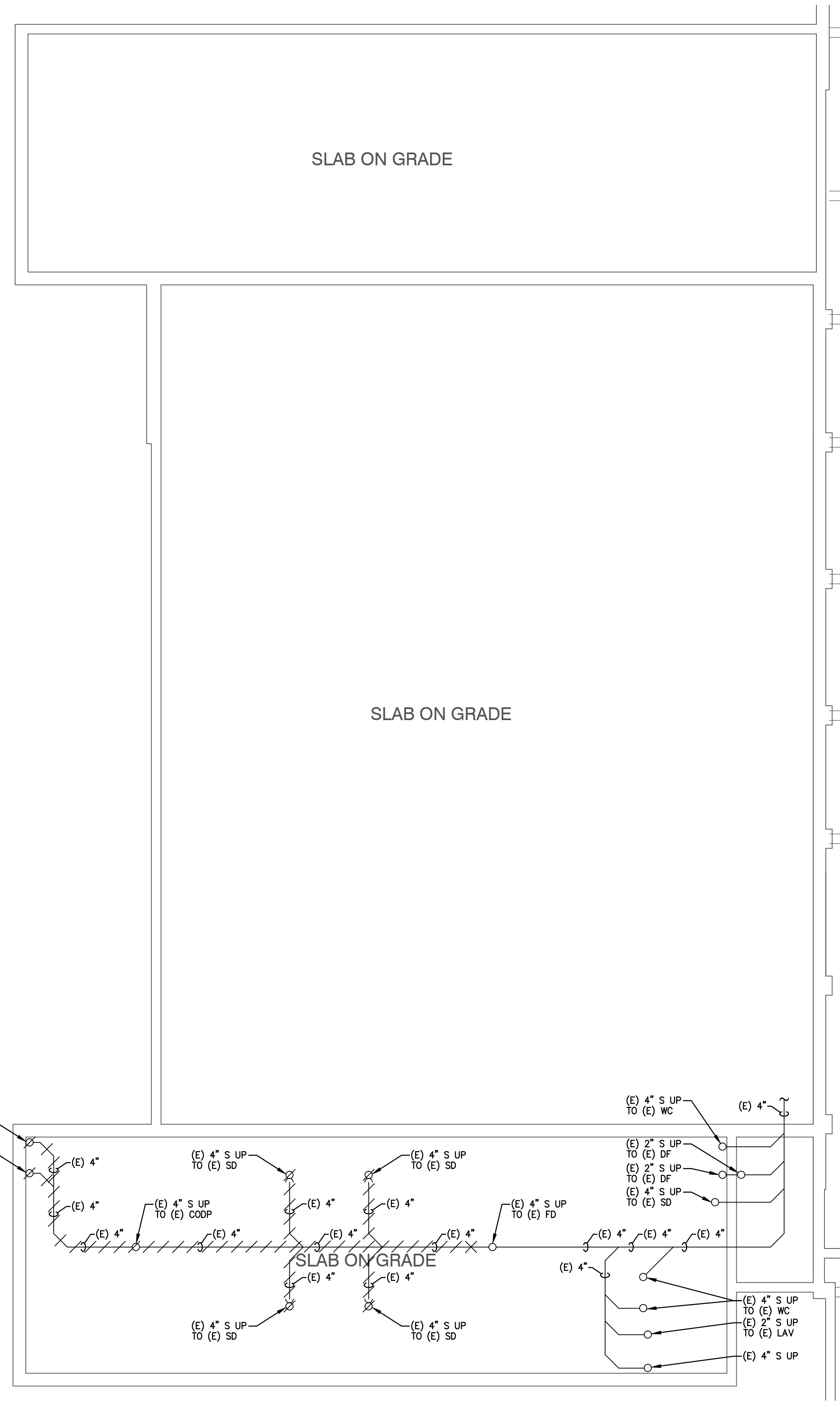
1 GYM FLOOR PLAN - PLUMBING DEMOLITION SCALE 1/8" = 1'-0" NOTES: 1. EXISTING SANITARY PIPING SHALL BE CUT BELOW FLOOR SLAB WHERE AND AS INDICATED.
